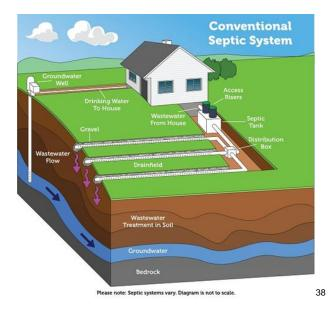
In a conventional OSTDS, a septic tank does not reduce nitrogen from the raw sewage. Approximately 30-40 percent of the nitrogen levels are reduced in the drainfield of a system that is installed 24 inches or more from groundwater in Florida.<sup>39</sup> This still leaves a significant amount of nitrogen to percolate into the groundwater which makes nitrogen from OSTDSs a potential contaminant in groundwater.<sup>40</sup>
