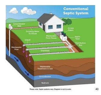
In a conventional OSTDS, a septic tank does not reduce nitrogen from the raw sewage. Approximately 30-40 percent of the nitrogen levels are reduced in the drainfield of a system that is installed 24 inches or more from groundwater in Florida.<sup>41</sup> This still leaves a significant amount of nitrogen to percolate into the groundwater which makes nitrogen from OSTDSs a potential contaminant in groundwater.<sup>42</sup>
